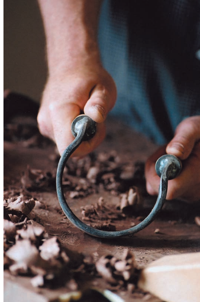
Left: The Oregon Black Walnut chair is a popular choice among Morrison's clients. Above: Morrison designed the Butterfly Joint specifically for his unique chairs. He uses the "Scorp" tool to, as he puts it, "scoop out a chair's seat."
